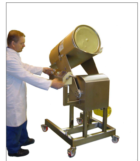
PalPharmaTip CBM100, similar to a CB100 but shown with self supporting mobile base
