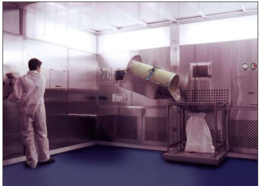
PalPharmaTip CB100, a study by a leading containment equipment manufacturer found that the use of an ergonomic drum positioner in a containment booth helped to keep the actual powder dispensing operator exposure level (OEL) many levels of safety below the accepted OEL using a time weighted average analysis, (TWA). Design available as an in line or cantilevered design depending on space constrictions.
