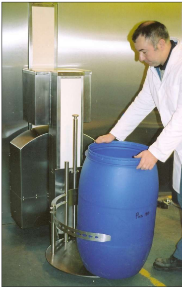
PalPharmaTip RR100, PLC controlled with the ability to rotate the drum in two orientations for dispensing powder to both a floor scale and a bench mounted scale
