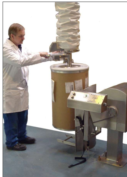
PalPharmaTip CB100, shown being loaded with the PalPharmaVac option for a complete ergonomic solution to powder dispensing and drum emptying
