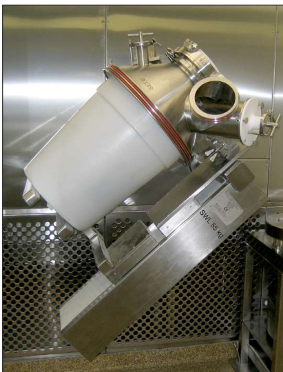
PalPharmaTip CBC100, similar to a CB100 but shown with the option to help the removal of empty drum liners in a contained method
