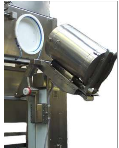
PalPharmaTip I100/2000, shown being used in conjunction with an isolator for highly accurate positional and docking requirements.
